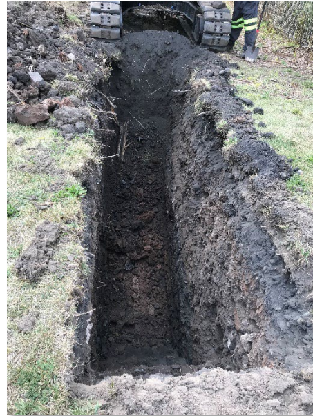
Breeze-rich fill also containing silt, rock, metal, wood, coal, coke, slag, and brick at TP-06-2020.
