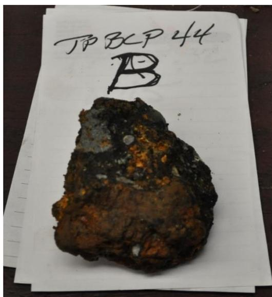
Photograph 4-16 – Slag Sample – TP-BCP-44
