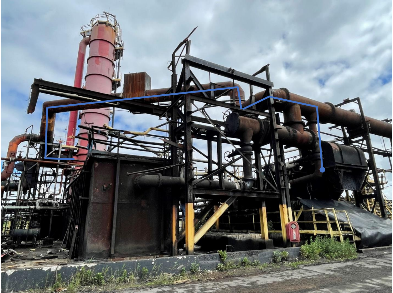
Photograph 3: The 30-inch line at base of primary cooler which connects directly to the tar decanter.
